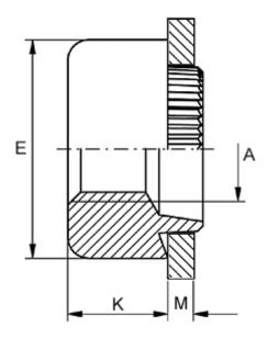
Female thread A = M3Height K = 3.0Outer diameter E = 6.0
